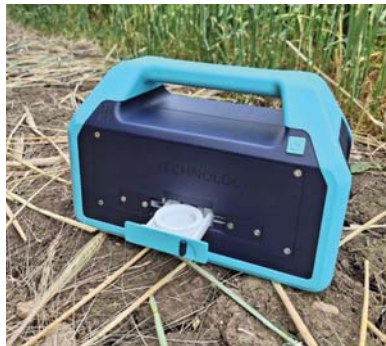
The hand-held and battery-powered PES device turns soil testing into a five-minute process.
